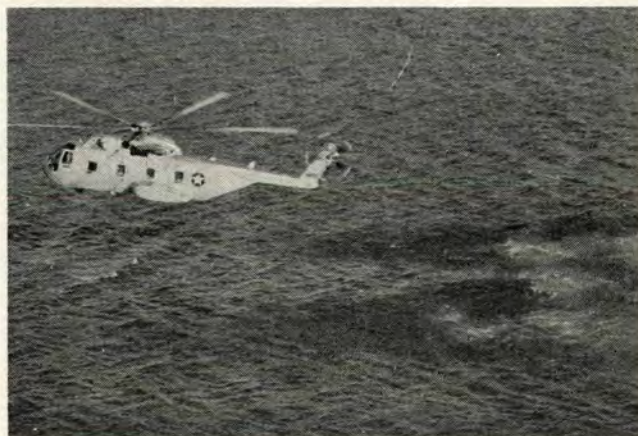
Effect of rotor wash is shown by disturbances on water below and behind helicopter.
